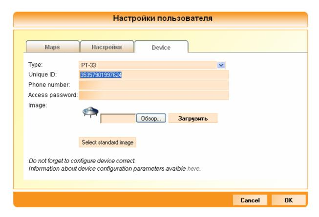
3. Now check that device is turn on, enable satellites and installed connection to server.
