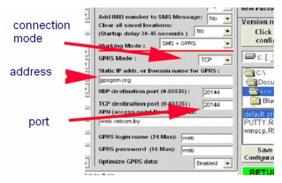
You can create this use the device configuration program, or send sms (some types of devices support this mode configuration).
